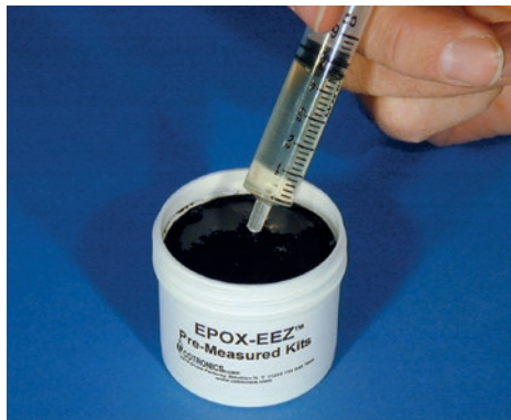
Dispense hardener into resin prior to mixing.
